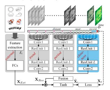
Fig. 3. ST-ResNet architecture. Conv: Convolution; ResUnit: Residual Unit; FC: Fully-connected.
