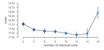
Fig. 13. Impact of network depth. We run each model 10 times where error bars show standard deviation.
