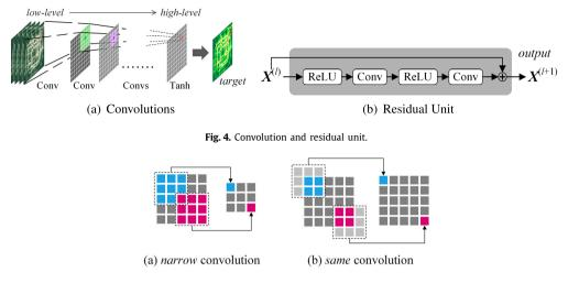
**Fig. 5.** Narrow and same types of convolution. The filter has size  $3 \times 3$ .
