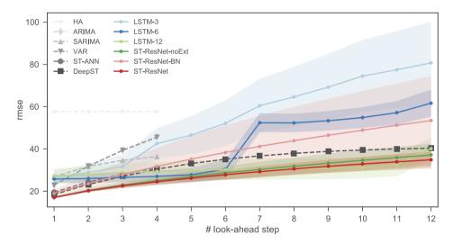
Fig. 18. Multi-step ahead prediction. For LSTM variants and ST-ResNet variants, we run each of them 10 times and use markers and shaded areas to denote mean RMSE and standard deviation, respectively.
